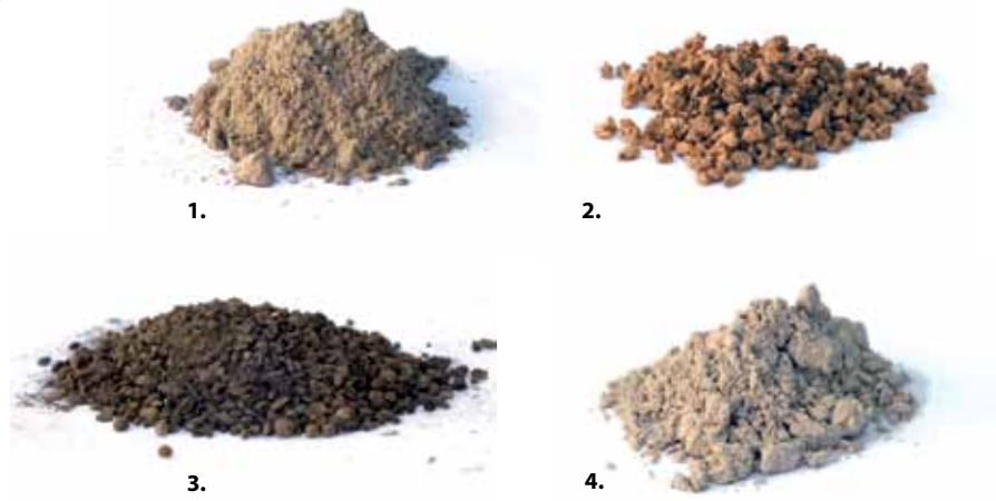
1. Diatomaceous earth / 2. Cork / 3. Clay / 4. Hydraulic lime
