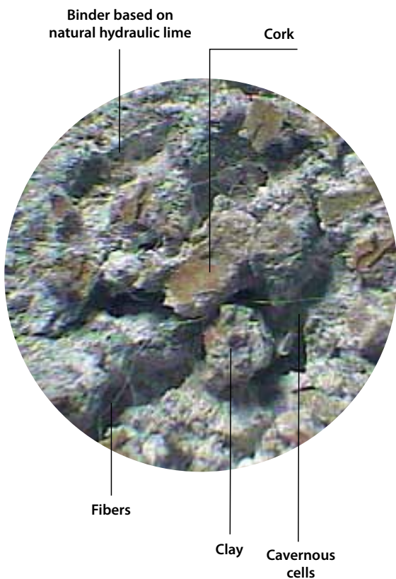
Diathonite Acoustix section (scaling to 200%)
